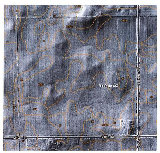
LIDAR is very intensive elevation mapping made with radar-like aerial photography. LIDAR usually provides the best image of a farm's topography. South and east-facing slopes are in shadow. West and north-facing are in sunlight in this image.
