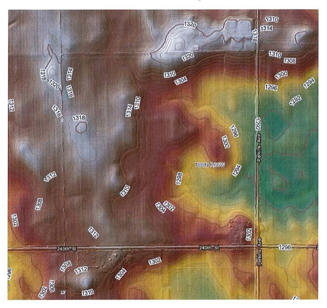
Elevation ranges from 1,318' on the west side to 1,292' on the east side, a change of 26' across one-half mile with an easterly slope.
