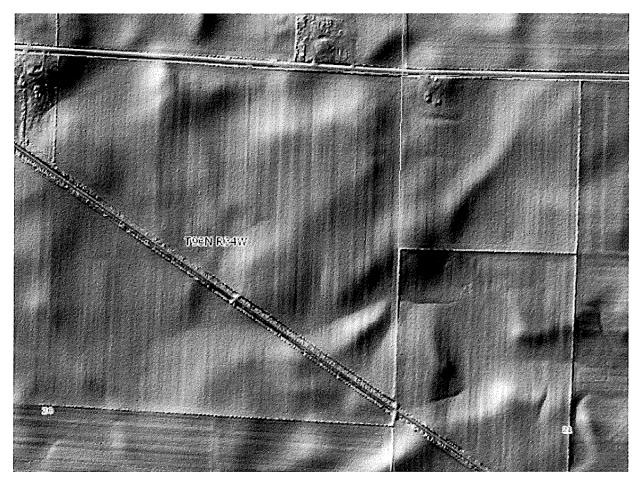
LIDAR (Light Detection and Ranging) is highly sensitive and intensive topographical mapping taken from specially equipped aircraft flown across the state of Iowa between 2007 and 2010. These maps show topographical features in much greater detail than can be noted on other maps or photos. LIDAR maps can be incorporated into GIS systems for construction projects or land management.
